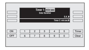
The count down of Timer 1 and 2 is shown in the lower area of the display.
